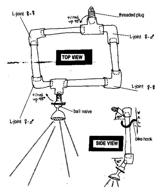
You cut the section of pipe into 2 14 inch sections and 2 12 inch sections and then connect all this stuff together with the plastic pipe cement as show in the diagram. Don't glue any of the threaded joints — the one on top is for filling and the one at the bottom is so you can remove the shower head assembly for cleaning, etc. What you have at the end of the process is a square of black pipe that holds about 2 gallons of water — enough for a 5 minute shower.
