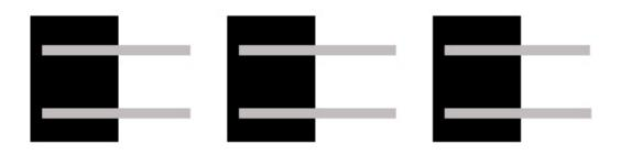
Next the extended piece of wiring is soldered to the back of the next cell as shown below.
